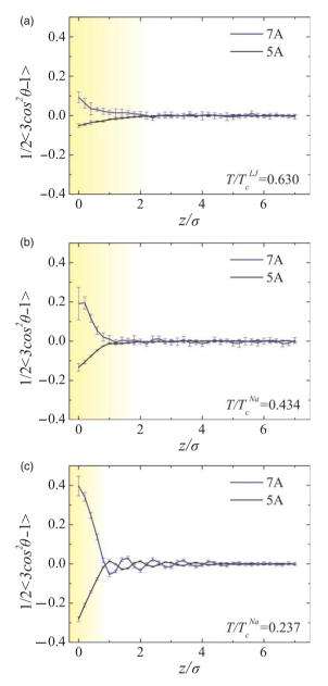
Figure 8. The ordering of the 5A and 7A clusters relative to the interface, as a function of the distance z from the interface. The angle  $\theta$  is the angle between the vector that connects the spindle particles and the normal to the surface. (a) Lennard-Jones, T=0.95,  $T/T^c = 0.880$ ; (b) sodium, T=0.542,  $T/T^c = 0.434$ ; (c) sodium, T=0.297,  $T/T^c = 0.237$ .
