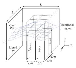
Figure 2. Identification of the position of a capillary perturbed interface. The interface is shown in blue and the cube is split into  $n^2$  columns *i*, *j*. The interface is assumed flat in each column and the position is extracted by a fitting step function (Equation (4)) to the columnar density profile  $\rho_{i,j}(z)$ . Note periodic boundaries apply in the *x* and *y* directions only.
