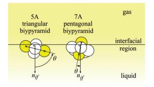
Figure 7. Definition of the orientational order parameter used in the case of the 5A triangular bipyramid and 7A pentagonal bipyramid.  $\theta$  is the angle between the normal  $n_{\rm if}$  to the plane of the interface (marked in blue) and the vector connecting the centres of the yellow spindle atoms.
