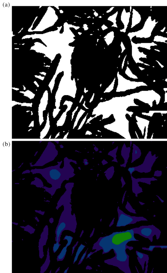
FIG. 4. (a) The thresholded and, so, binary image produced by image analysis of the area in the white box in Fig. 2. Fiber voxels are in black and air voxels are in white. (b) Heatmap of the z component of velocity in the same area. Again, the black region corresponds to the fabric. The dark purple, blue, and pale green regions correspond to velocities less than the mean, between the mean and ten times the mean, and over ten times the mean velocity, respectively. The area of both images is 594 \times 504 \mu\text{m}^2 .
